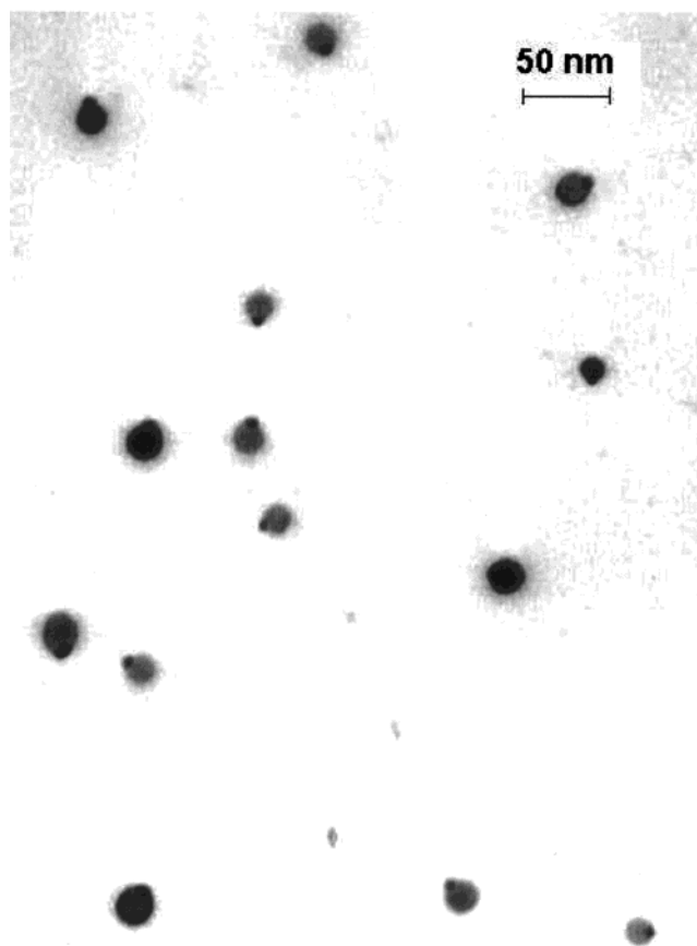
Figure 4. Transmission electron microscopy image of the silver nanoparticles obtained via chemical reduction using 1 as the template.
